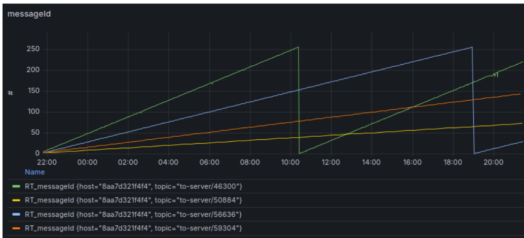
Figure 17: Large messages of 1014 bytes are sent from three nodes in the LoRa mesh network (id 46300, 50884, 59304) for 24 hours to a gateway node (id 56636). Sending periodicity: node 46300 every 3 minutes, node 50884 every 20 minutes, node 56636 every 5 minutes, node 59304 every 10 minutes. The MessageId values are obtained from a subscription to the MQTT broker.
