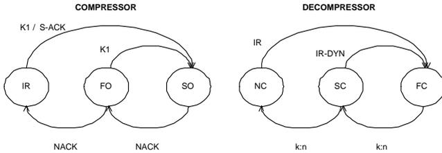
Figure 3: Compressor and decompressor state-machine.
