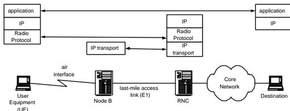
Figure 1: UMTS Architecture (air interface and radio access network).
