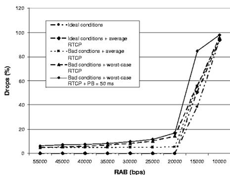
Figure 7: RoHC: Packet drops vs. bandwidth.
