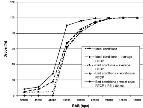
Figure 4: No RoHC: Packet drops vs. bandwidth.
